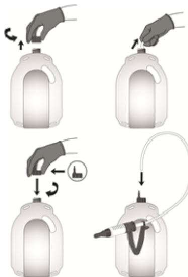
Figure 2 Attaching the recommended dosing gun to the 2.5 and 5 litre containers:
