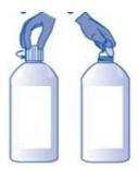
3) Remove the protector cap from the tip of the nozzle of the pump.
