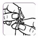
**Step 2:** With the other hand, press downwards on the smaller disk until the 2 disks meet evenly. This will pierce the seal.
