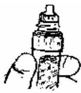
Unscrew outer and inner seal caps to expose wire prongs.
